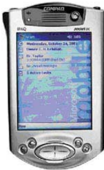
Figure 31. iPaq 3870 with Pocket PC 2002 operating system and 206Mhz Intel StrongARM 32bit RISC Processor.
