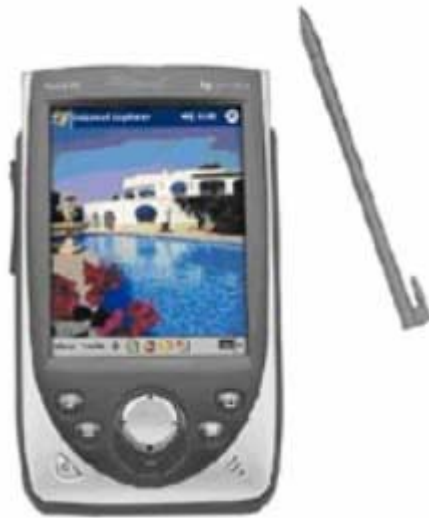
Figure 30. HP Jornada 568 handheld computer with Pocket PC 2002 operating system and active matrix screen.
