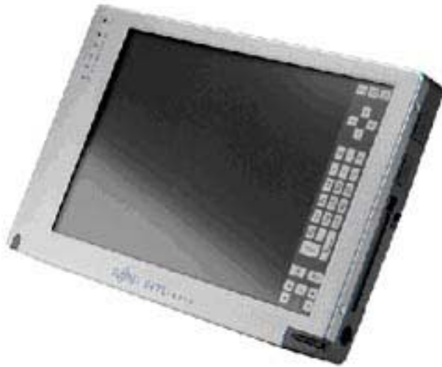
Figure 32. Fujitsu Stylistic LT P-600 is a tablet computer with 800 x 600 true color display.
