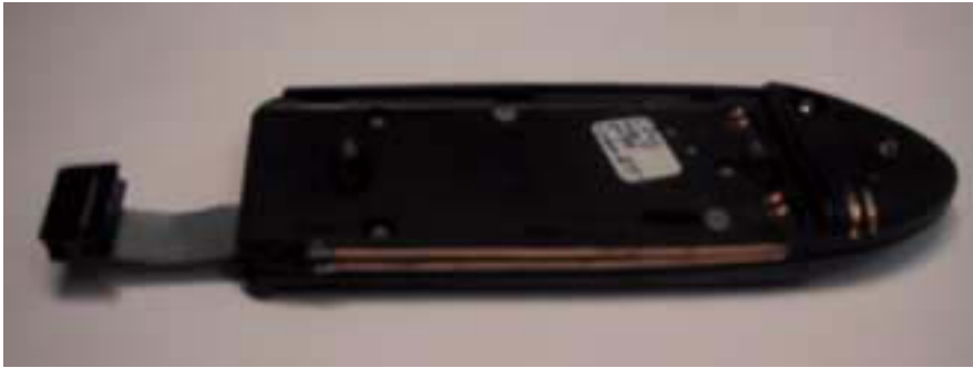
Figure 6. Sensor box for examining context-awareness of mobile devices.
