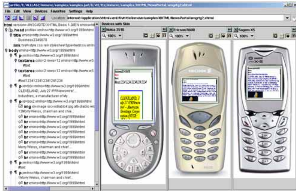
Figure 7.9. XHTML document simulated in various kinds of simulator configurations. UAProfs and style sheets are used in presenting the content.
