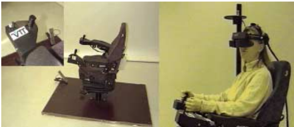
Figure 39. Simulator system for analysis of the sitting operation used in the case studies 2 and 3.
