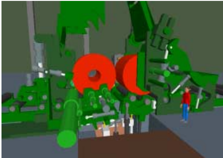
Figure 29. A view of the coilbox machine in the 3-D model used for the safety analysis.
