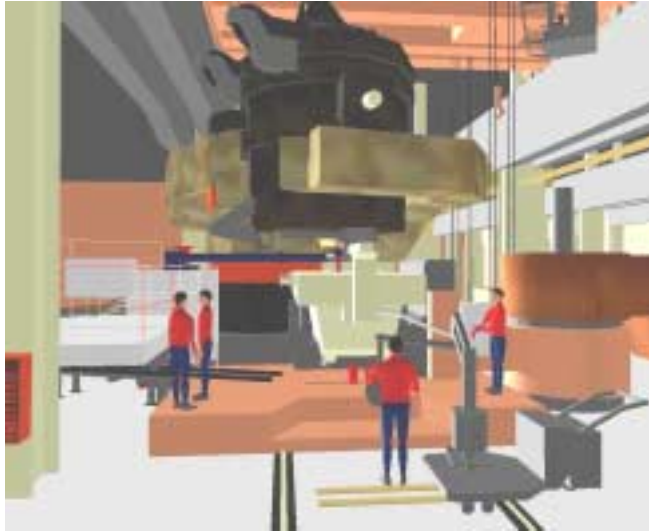
Figure 27. A view to the continuous casting machine with the 3-D model used in the safety analysis.
