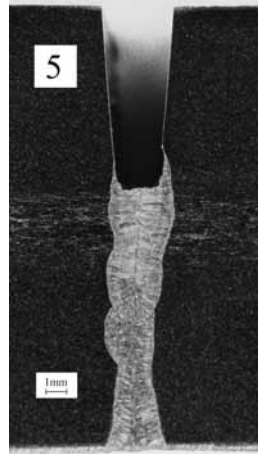
Figure A7-5. The set-up and cross-section of testpiece 5. in the TAGUCHI experiments for the first filling pass with hybrid welding. Parameters in Appendix 4.
