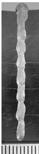
Figure 4.17. The cross-section of the weld with a plate thickness of 35 mm. Testpiece 2 with 8 passes. Parameters in Appendix 3.
