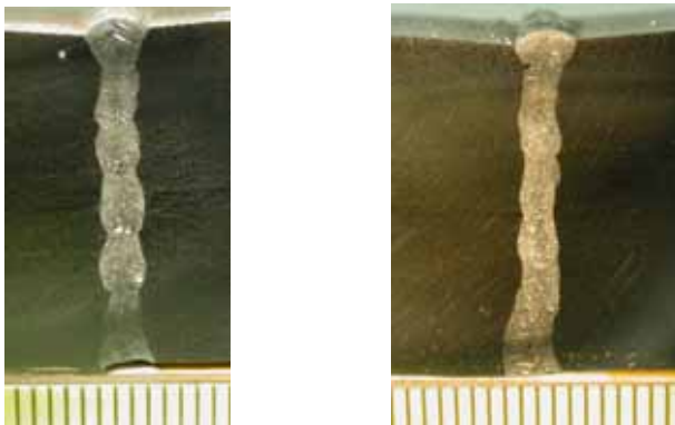
Figure 4.16. Cross-sections of the welds with a plate thickness of 20 mm. On the left hand testpiece 2. with 5 passes and on the right hand testpiece 3. with six passes. Parameters in Appendix 2.
