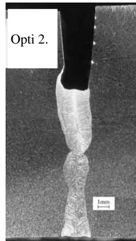
Figure 4.21. The set-up condition and cross-section of the first filling weld made with hybrid weld. Parameters in Appendix 4.
