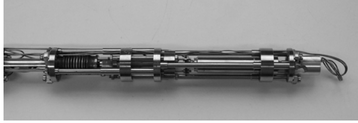
Figure 5.1: The in-reactor tensile test module together with instrumented irradiation rig is lowered in the core of BR-2 test reactor.
