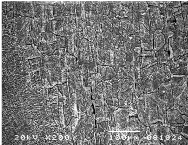
Figure 59. General and grain boundary dissolution close the weld / base metal 1 fusion line in irradiated HAZ specimen. No heat treatments.
