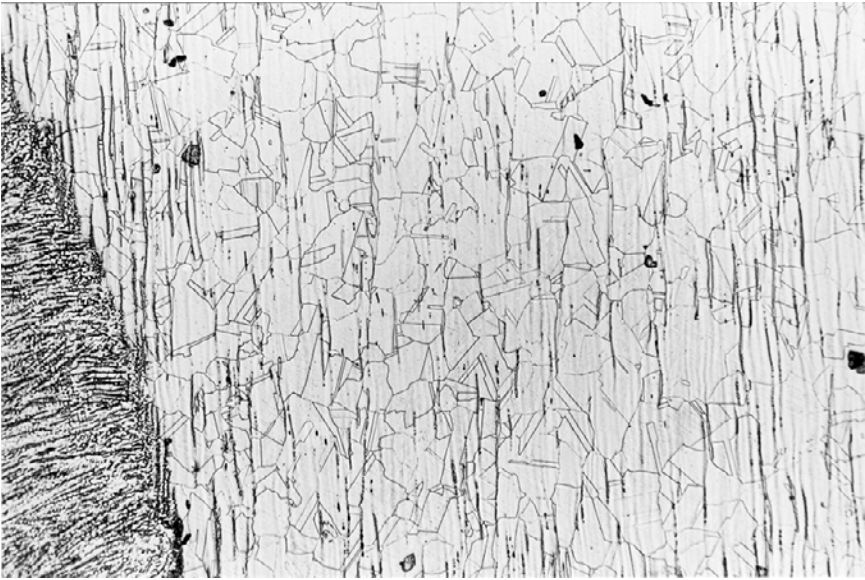
Figure 31. The microstructure of non-irradiated base metal 1 close to the weld fusion line. The matrix contains large \delta -ferrite lamellas (100x).
