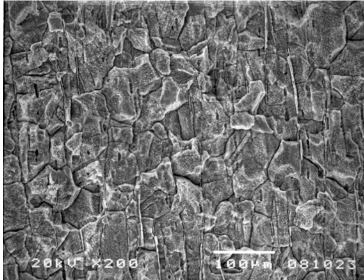
Figure 58. General and grain boundary dissolution about 1.5 mm from the weld / base metal 1 fusion line in irradiated HAZ specimen. \delta -ferrite dissolution was minimal. No heat treatments.
