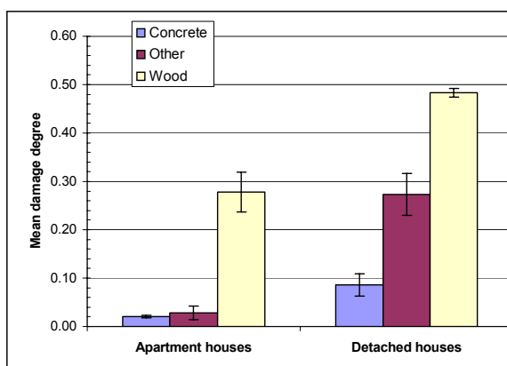
Figure 59. Mean damage degree in apartment and detached houses. The numbers of observations are similar to Figure 60. The error bars represent the standard deviation of the mean (see Section 2.7).
