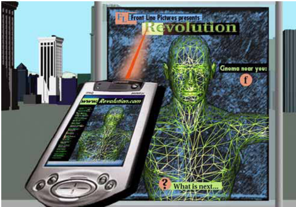
Figure 41. Pointing could be used to extract information about the surroundings. The picture presents a movie poster with embedded tags. Based on the tag information, the mobile device can download a corresponding URL to the device. [VAL]
