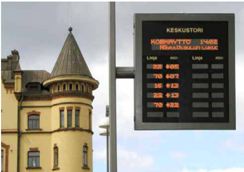
Figure 1. A display for arriving buses at a bus stop. The dynamically updated times of arrival present context-awareness. The information is also location-specific.
