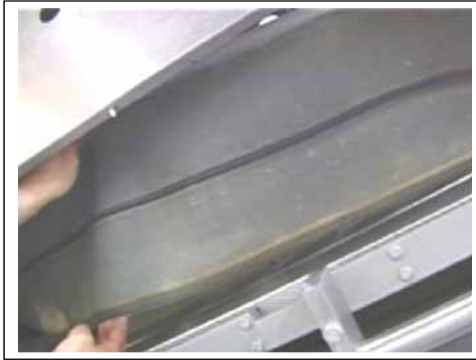
Figure 15.10. The underside of the conveyor belt. The conveyor belt is not easy to dismantle, as it should be and it is virtually impossible to clean underneath.
