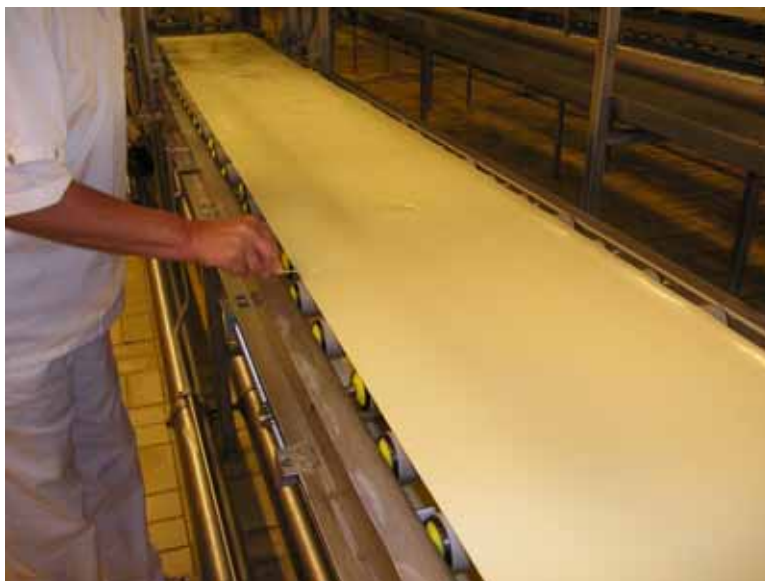
Figure 7.2. A critical spot contaminated with fungi was found under the conveyor belt.
