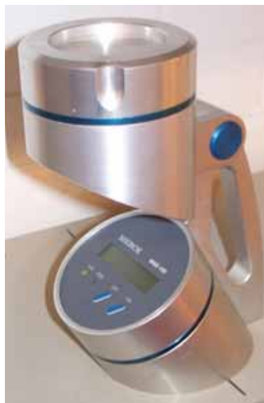
Figure 3.2. The MAS-100 air sampler is an impactor.
