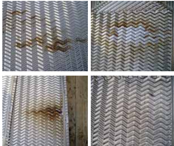
Figure 15.8. Visual inspection of a plate from a Pasteur used for 5 years.
