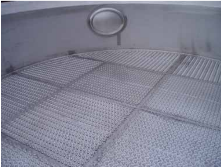
Figure 15.2. The perforated sheet above which the powder is kept suspended.
