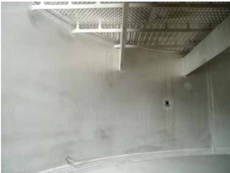
Figure 15.3. The underside of the perforated sheet in the static fluid bed including bearers. Note the cross bearer above the supporting bottom bearer.
