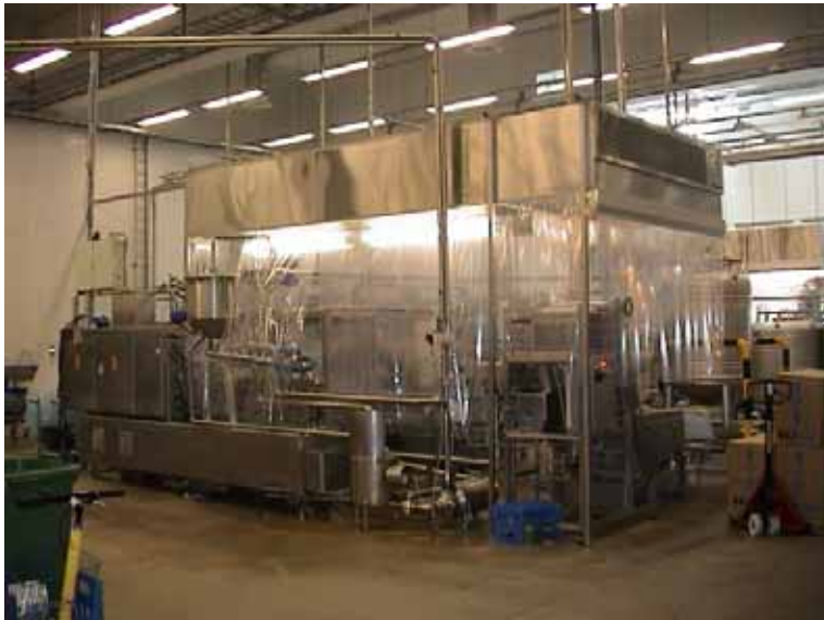
Figure 5.2. Doso-packing machine with HEPA filters installed. The whole filling space has been protected with a plastic cover.
