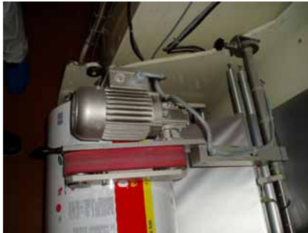
Figure 15.14. The level sensor that ensures the correct powder level in the funnel. If the sensor is removed, it can be refitted in several ways. If it is fitted incorrectly, the rotating snail may hit the level sensor and break off metal, which is mixed into the powder. This should not happen. A safety device, which is extremely easy to construct, must be installed to ensure that the level sensor is fitted in the correct position.
