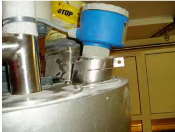
Figure 15.13. The geared motor, which is located in the middle of the powder funnel. If a leak develops in the gear, oil will seep into the powder and therefore pass on to the consumer. Due to this, it is necessary to redesign the bag filler so that the gear is located outside the powder funnel. The gear must have a collecting tray on which any oil leaking out of the gear is collected so that it cannot run down inside the foil into the bag.
