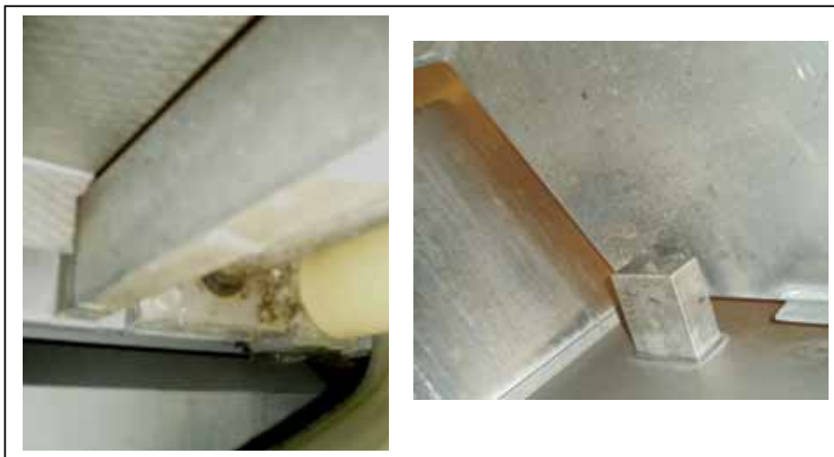
Figure 15.11. The access to the far corners inside the slicer is awkward and the corners are therefore not cleaned properly.
