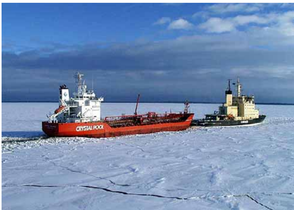
Figure 5. Icebreaker assisting a chemical tanker in the Gulf of Finland (photo: Finnish Maritime Administration).
