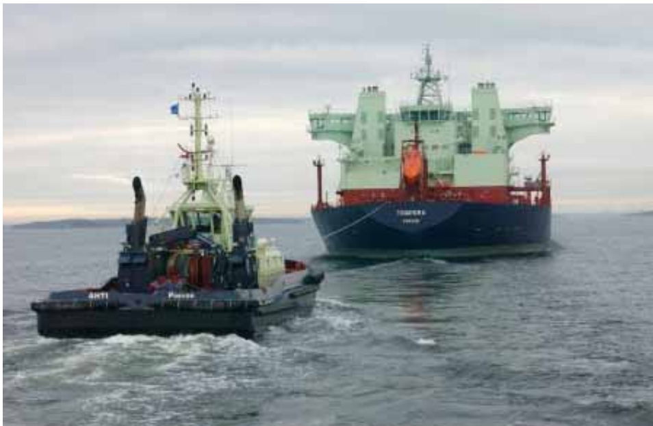
Figure 40. New escort tug boat Ahti assisting DAT-ship Tempera on her way to Sköldvik oil terminal. MT Tempera is built in 2002 and has 1A Super Ice Class.
