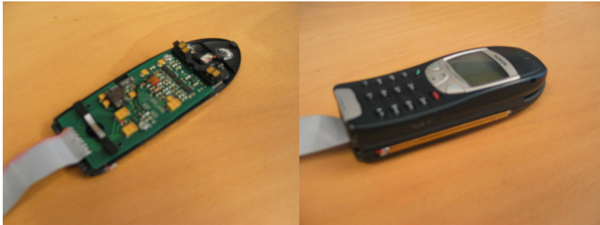
Figure 4.3. Sensor-box module and module attached to the back of a mobile phone.
