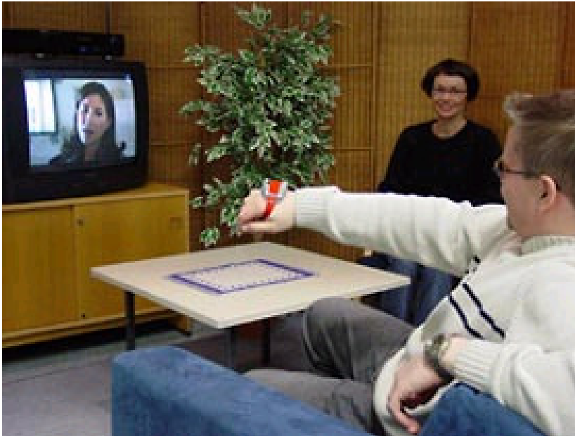
Figure 4.22. Controlling a TV-set with gestures. The SoapBox is in the casing on the back of the hand.
