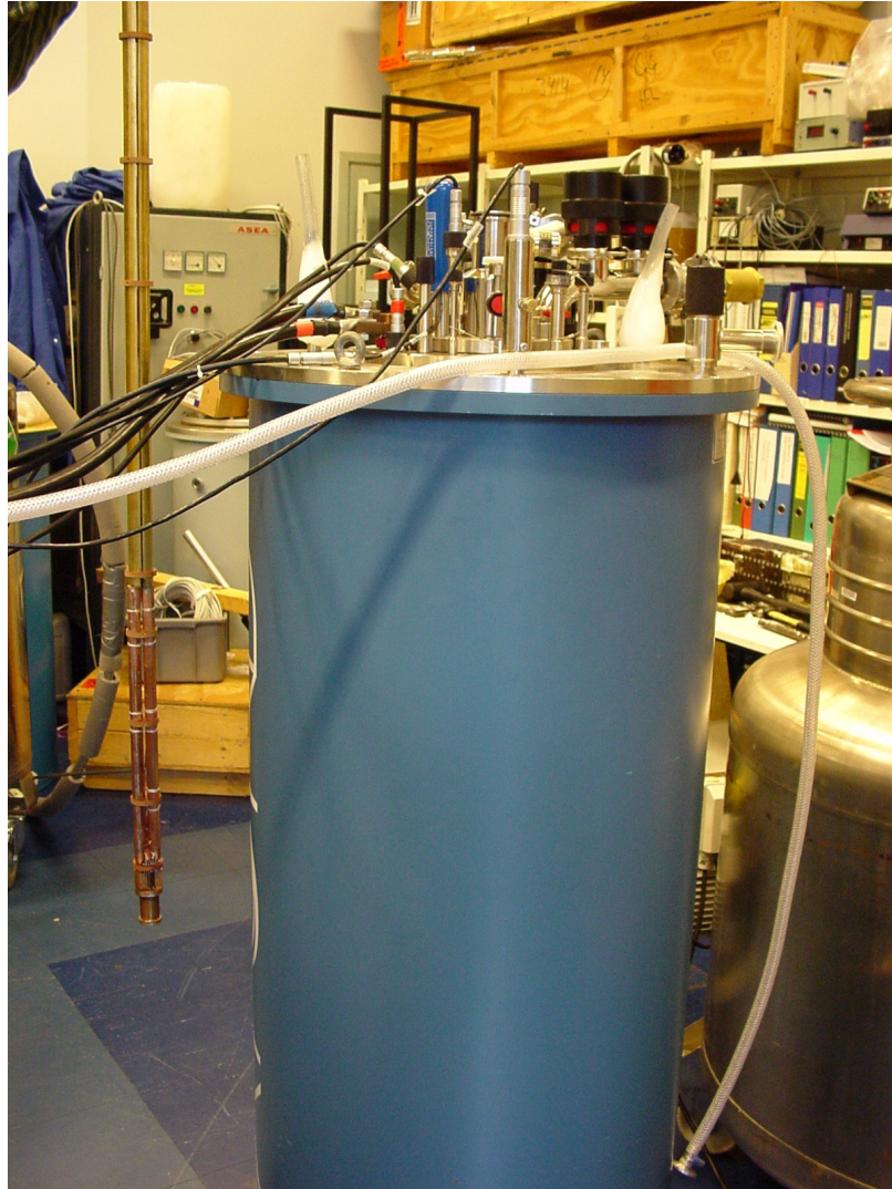
Figure 6.24: The sample holder used in the benchmarking tests of the Nb 3 Sn strand.
