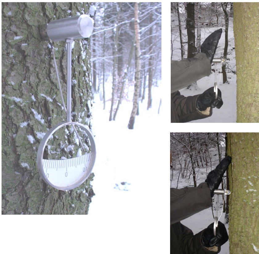
Figure 4. The S-GAG – an instrument used to determine the spiral grain angle on coniferous trees.
