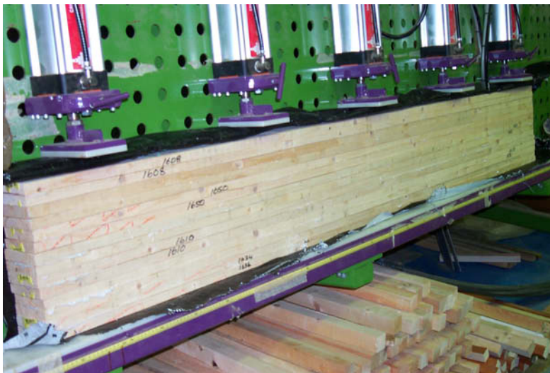
Figure 22. Re-engineered battens being pressed.
