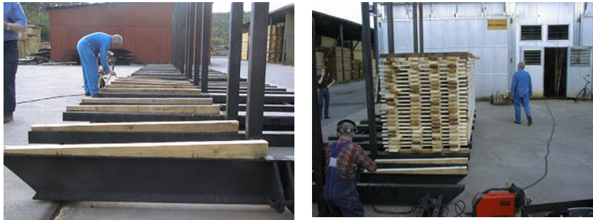
Figure 47. Inclined supports on a timber wagon (left) and a stickered kiln stack (right). From drying tests performed by SP Trätek.
