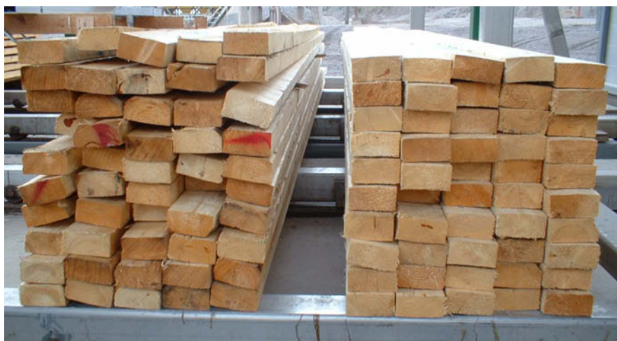
Figure 33. Unloaded and loaded battens after drying.
