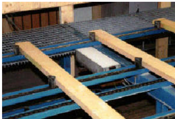
Figure 14. FMI Sensor of capacity type moisture content meter manufactured by Brookhuis.
