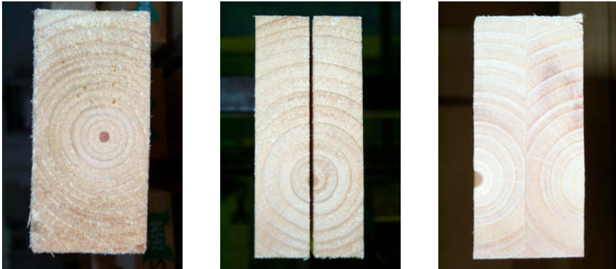
Figure 21. Boxed pith batten, split along its length & bonded in a “back to back” orientation.
