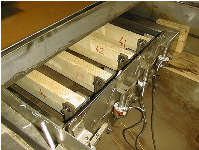
Figure 48. Twisting of timber during laboratory kiln drying at SP Trätekt in Sweden. Direction of pre-twisting is opposite to the natural direction of twist in timber.
