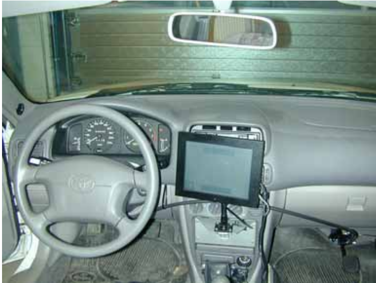
Figure 11. The touch screen used for the visual task mounted in the instrumented car.
