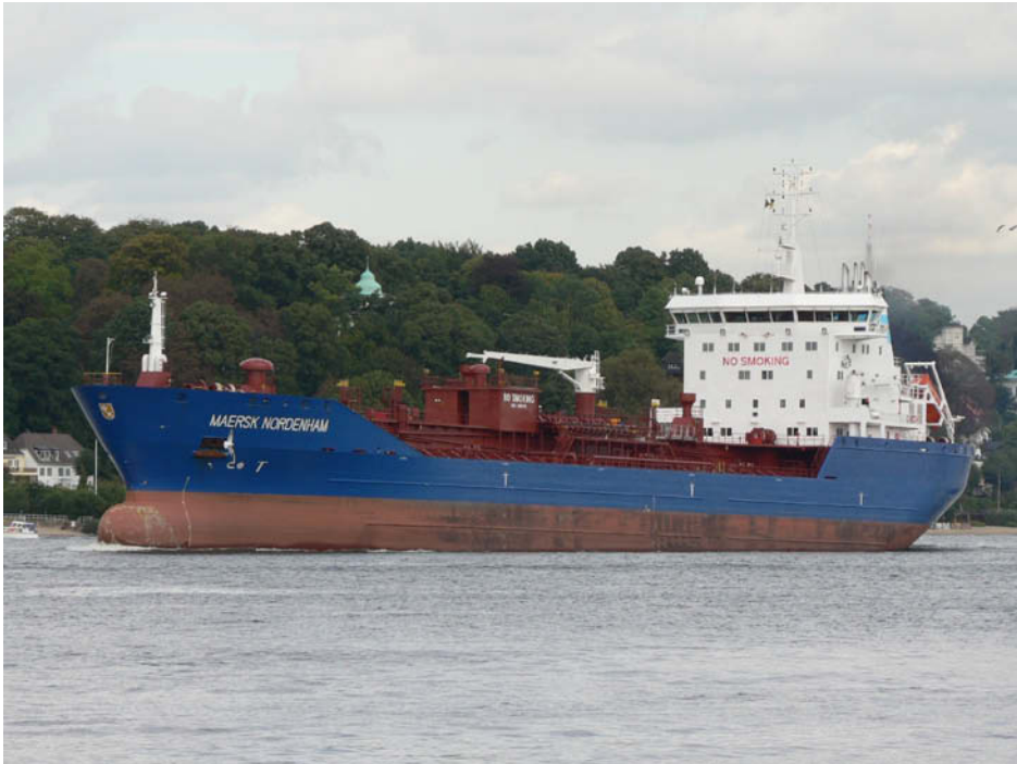
Figure 3. Maersk Nordenham – a typical chemical/oil products tanker, 16,716 dwt. Photograph courtesy of Schindler, 2005.
