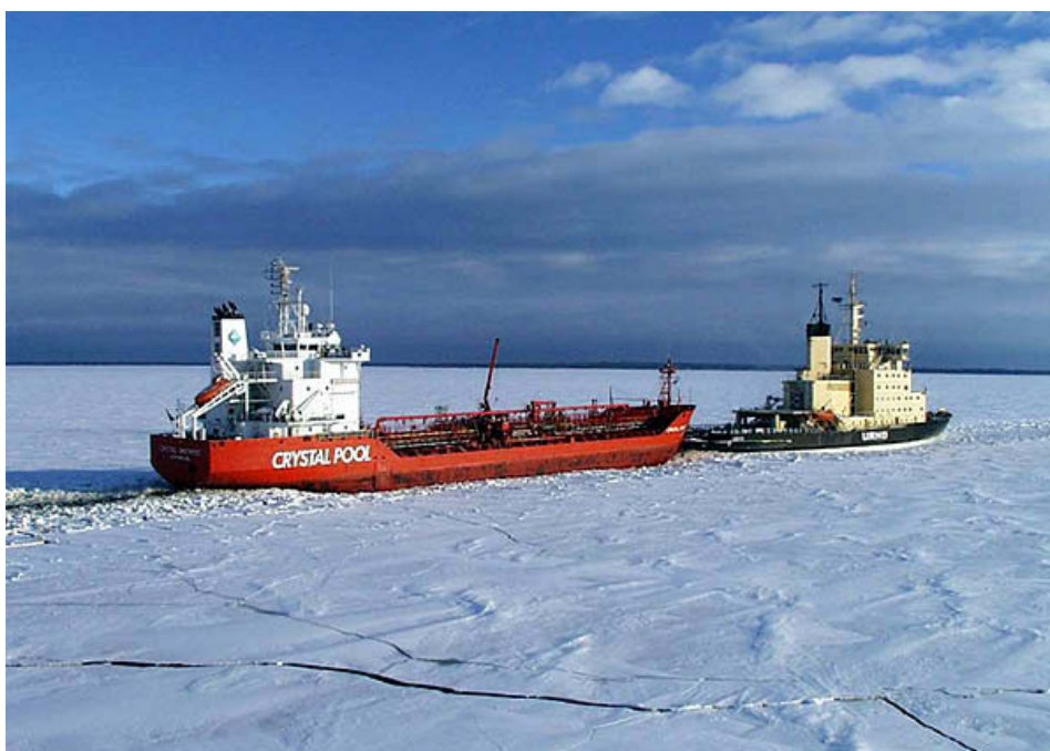
Figure 17. Icebreaker Urho assisting a chemical tanker in the Gulf of Finland. Photograph courtesy of Finnish Maritime Administration.
