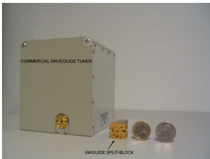
Figure 12. A photograph of a motorized waveguide impedance tuner and a waveguide split-block.
