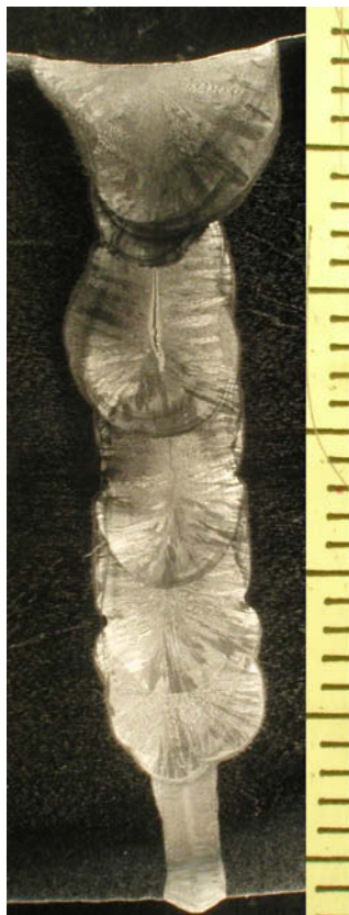
Figure 5.5: Macro cross-section of multi pass test weld and used groove geometry. On the right: Obtained vertical groove fill-ups for the each filling pass. Used variable parameters: welding speed 0.3–0.4 m/min, focal position +25–+40 mm, wire feeding rate 13.5–16.5 m/min.
