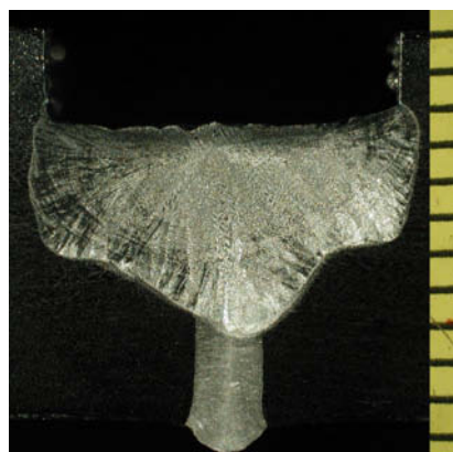
Figure 5.4: Macro cross-section of test weld and used variable parameters. The used gap width: 10.8 mm.
