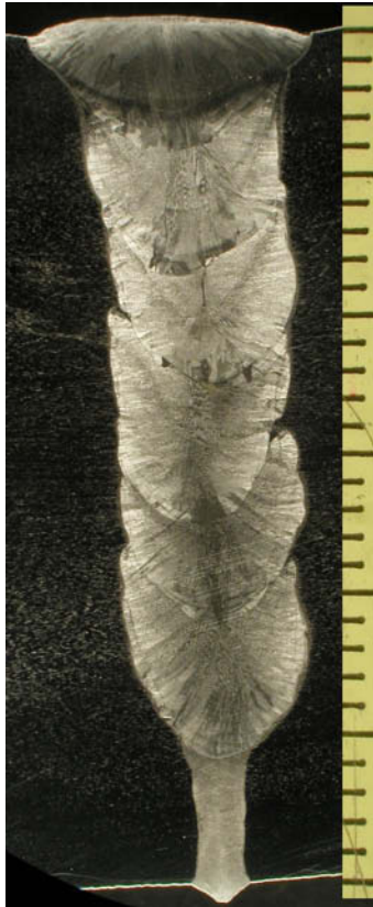
Figure 5.6: Macro cross-section of multi pass test weld and used groove geometry. On the right: Obtained vertical groove fill-ups for the each filling pass. Used variable parameters: welding speed 0.3–0.35 m/min, focal position +40–+45 mm, wire feeding rate 13–16.5 m/min.
