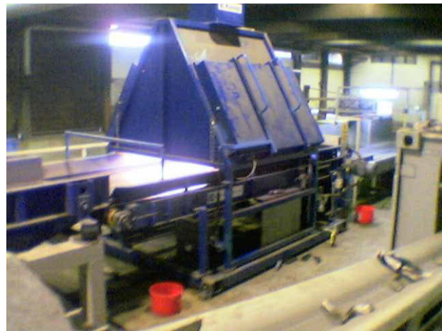
Figure 1. The sorting machine Kombi with inductive and colour camera sensing systems
