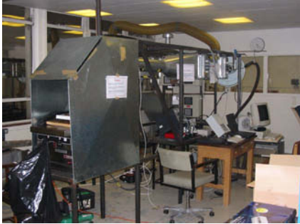
Figure 7. Test rig which simulates industrial hood system
