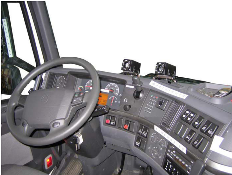
Figure 2. The FaceLab system setup in the test truck
