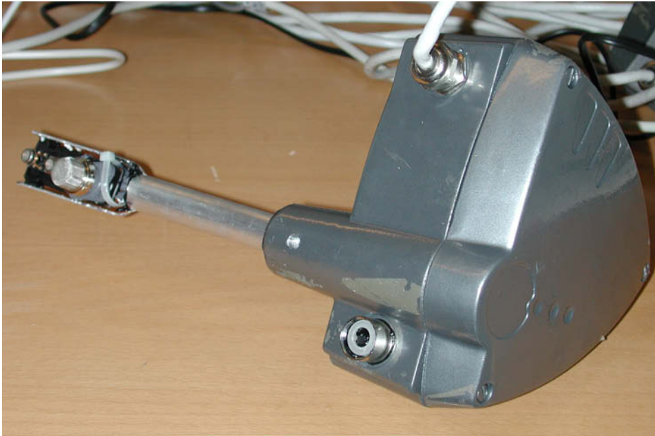
Figure 4. The developed data acquisition device for detecting gas concentrations in Publication IV.
