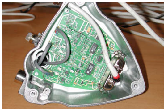
Figure 1. Electronics of the sensor device in EMC protected enclosure
