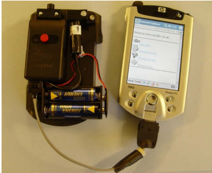
Figure 4. The Physical Browser components: iPAQ (right), with the embracing sleeve removed (left). The sleeve contains a central SoapBox, laser beam unit, and batteries. The SoapBox has a pointing button (shown red in the middle of the SoapBox) to activate the laser unit and the IR transmitter. The nozzle around IR led is pointing out from SoapBox.
