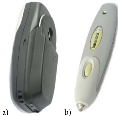
Figure 2. Nokia 6600 phone with RFID reader attached (a) and a Bluetooth barcode reader pen (b).
