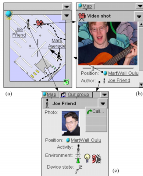
Figure 3. Screenshots describing a scenario in which Joe has recorded a short video clip of a stand-up comedian and placed the document on the map. Arrows between screens describe navigation achieved by clicking at the starting point of the arrow.
