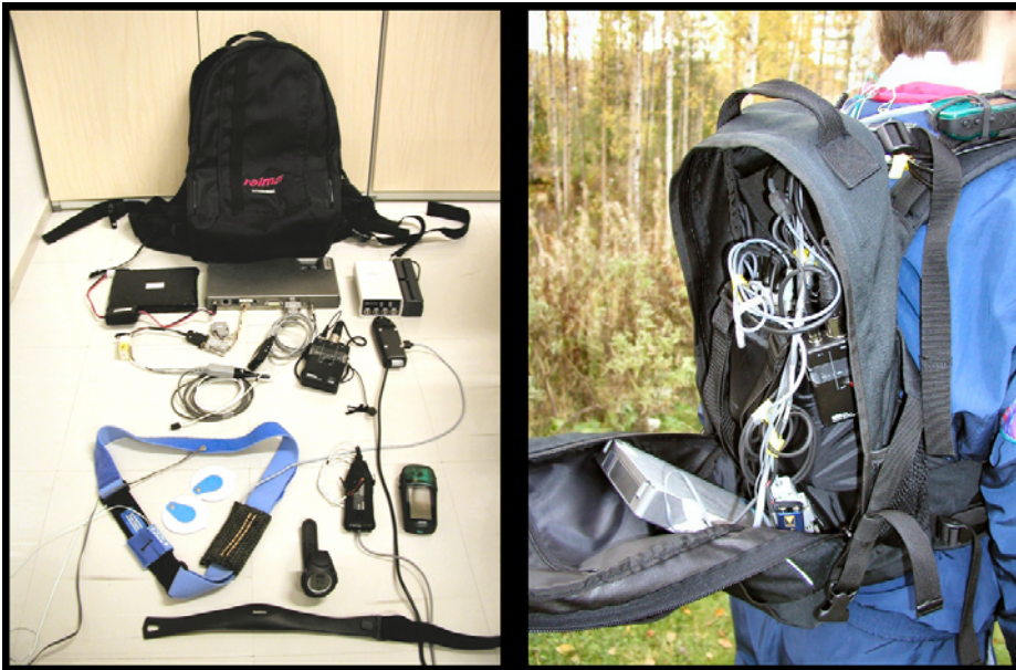
Figure 1. Palantir Data Acquisition System: Left: equipment on the floor, Right: equipment in the rucksack. Left, topmost row: Rucksack. Second row: PC battery, PC, Embla recorder (white) and battery. Third row: Oximeter (gray), SoapBox (black), microphone and amplifier (black), SensorBox. Fourth row: Respiratory effort strap (blue), body position (blue, around strap on the left), ECG electrodes (white-blue), skin temperature (silver, on top of blue strap), skin resistance (gray, around blue strap), Suunto wrist-top computer and its heart rate strap below, second oximeter (black), GPS navigator.
