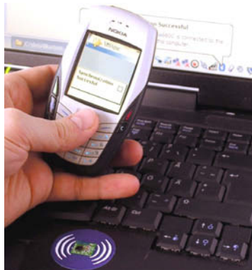
Figure 7. SMS messages are sent to the PC by touching the RFID tag.
