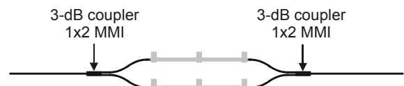
Fig. 2 Mach-Zehnder Interferometer with two 3-dB 1x2 MMIs. The grey areas represent the heaters.
