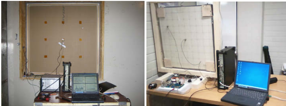
Figure 128. Measurement set-ups for transmission loss and EMA-actuator measurements.
