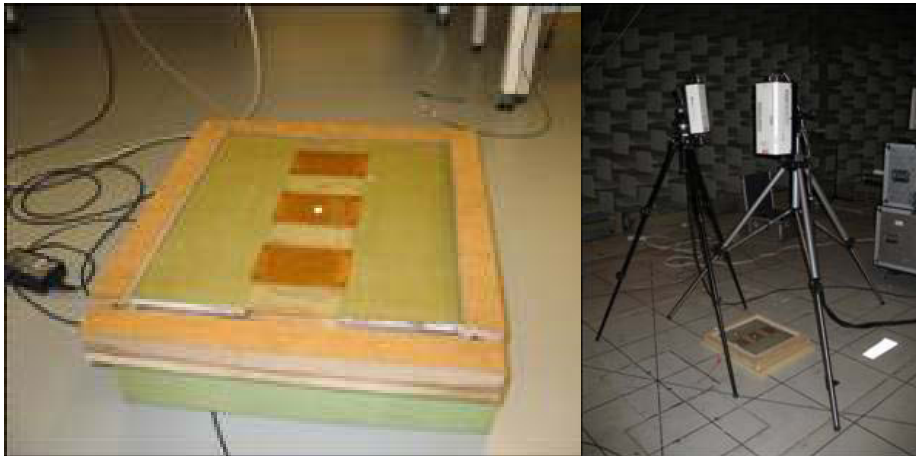
Figure 119. Piezocomposite actuator based on three MFC actuators. Dynamic behaviour of the element was measured with laser vibrometrer.
