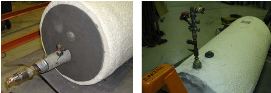
Figure 77. The prototype of a modular PCM cool storage with water inlet/outlet port ready for test measurements.
