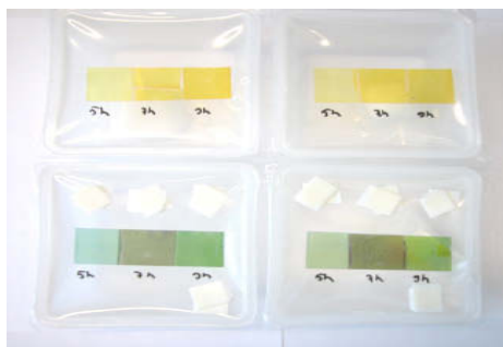
Figure 22. Testing indicator substances for freshness indicators.
