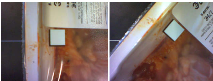
Figure 23. Coloured squares attached to a food package. The pictures are taken with a camera phone. The imaging distance is 6 cm. In the right the camera phone is twisted 40 degrees.
