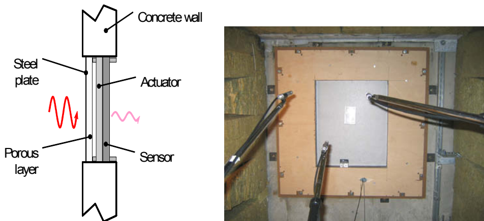
Figure 126. Scheme of the test setup for the testing of active sound insulation of a car sound package mock-up (left) and the evaluation microphone positions approximately at 1 m distance from the sensor panel on the receiving side (right).
