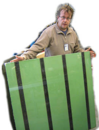
Figure 118. Striped panel and the improvement of sound transmission loss of striped panel compared to reference panel.
