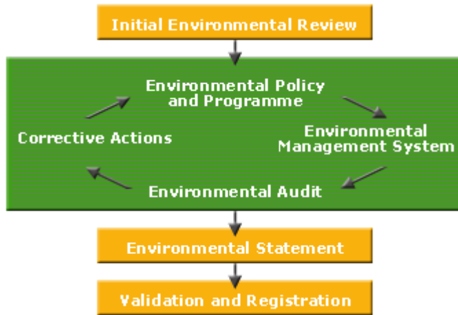
Figure 6. The core of the EMAS scheme described with help of the so-called "continuous improvement circle".
