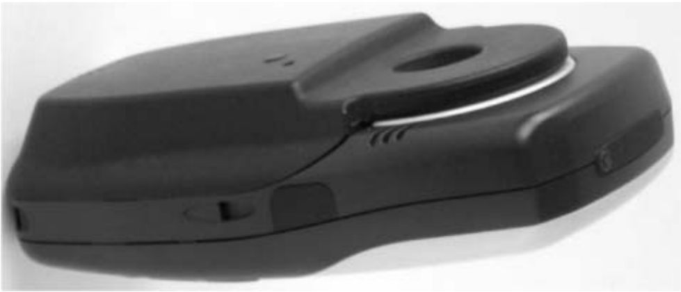
Figure 4.4 RFID reader attached to the back of a Nokia 6600 phone.
