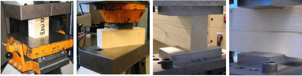
Figure 11. Perpendicular to grain tests. From left to right: EN408, ASTM D 143, beam end, and continuous beam.
