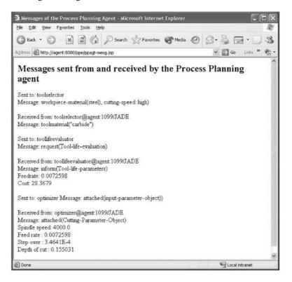
Figure 8 Machining process verification
