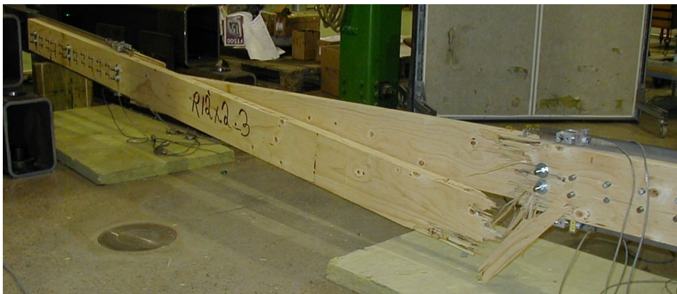
Figure 11. Failure, which has occurred across the specimen.
