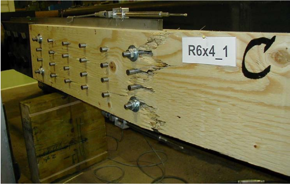
Figure 8. Failure by tension at the farthest column of dowels.
