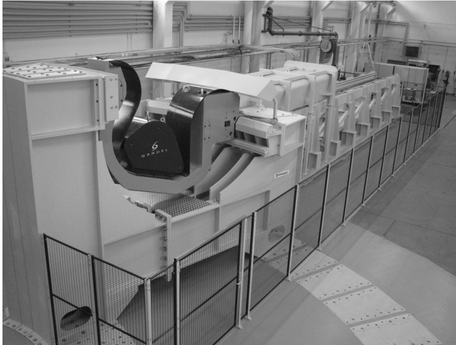
Figure 4.5: DTP2 Divertor Region Mock-up stage 1.
