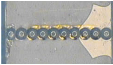
Figure 48. A double-sided microlens array on top of the LTCC substrate having a VCSEL array flip-chipped on the other side. The active areas of the VCSELs are seen through the lenses and LTCC via holes.
