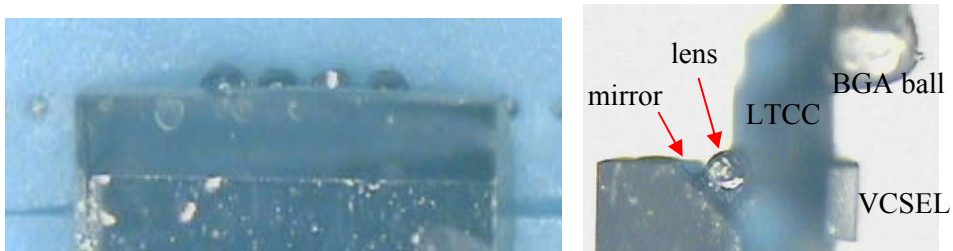
Figure 43. Micrographs of ball-lens-based coupling component mounted on the Tx module substrate having a VCSEL array on the other side; (left) viewed from the rear of the coupling component; (right) side view, where only one ball-lens can be seen.
