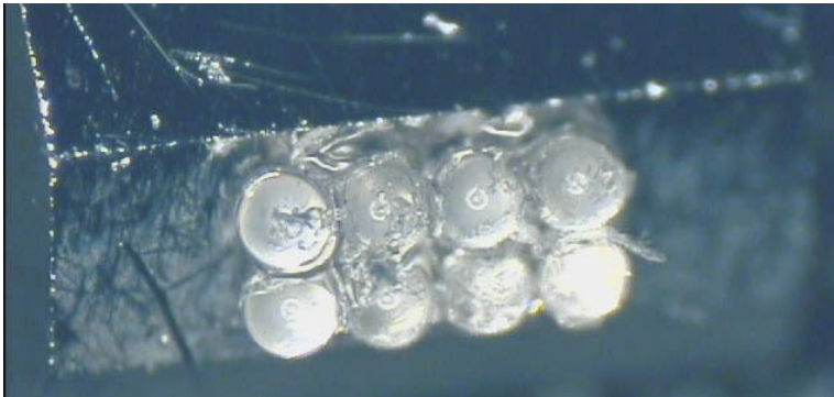
Figure 42. Micrograph of micro-ball-lenses glued onto an aluminium-coated bevel of a glass substrate.
