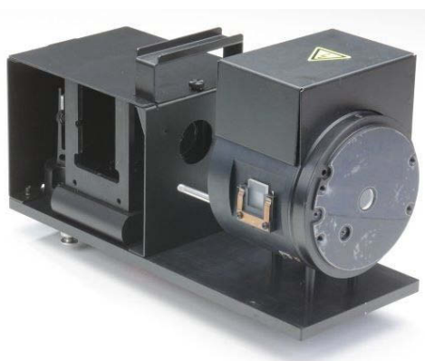
Figure 2. DRA-2500 integrating-sphere accessory for Varian Cary 5000 spectrophotometer.
