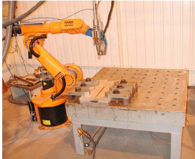
Figure 4.7. The lay-out of the experimental set-up: Laser-arc-hybrid welding head attached to the KUKA-robot's wrist flange. Rigid 170 mm thick table with clamping system.
