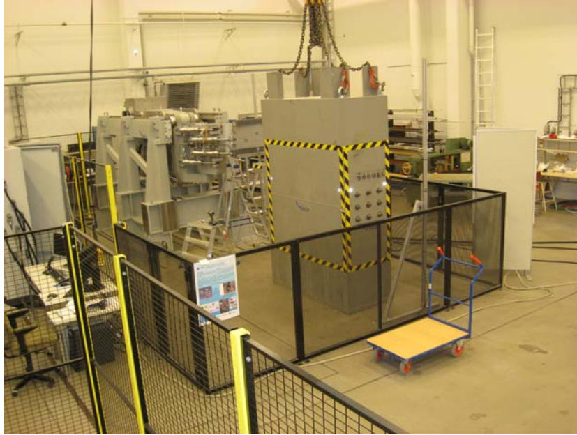
Figure 4.6. Safety system of the test rig.
