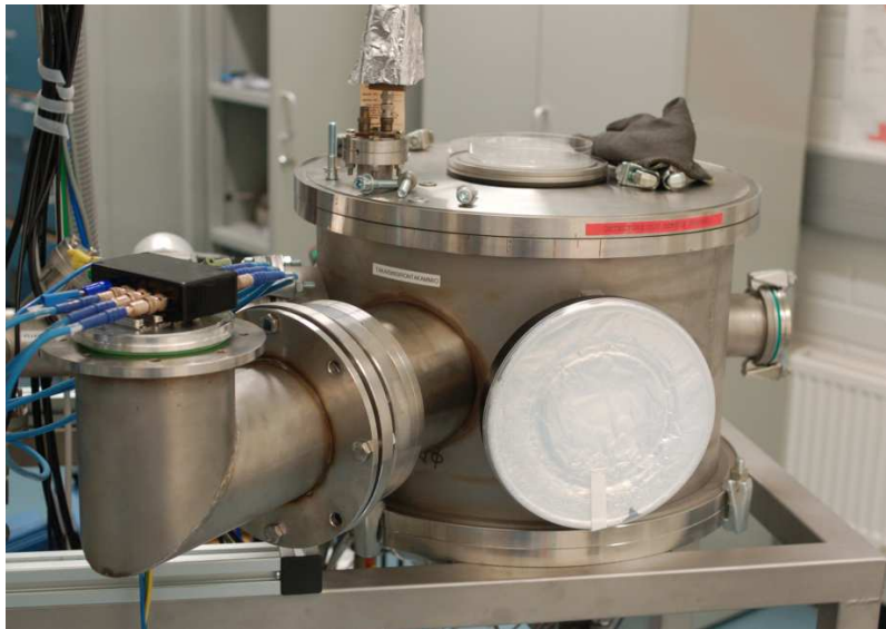
Figure 3.22. Rutherford backscatter chamber used for the beam tests. The test setup has been installed to the front-left port
