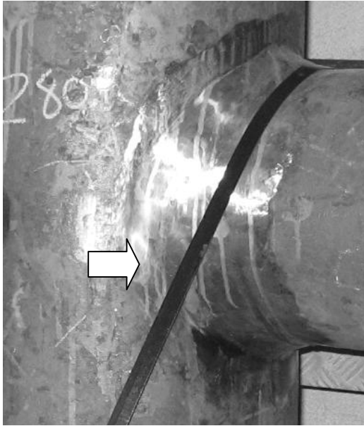
Fig. 1. A) Upper nozzle of high pressure mixer. B) Detail of 200 mm crack at nozzle weld (HAZ).
