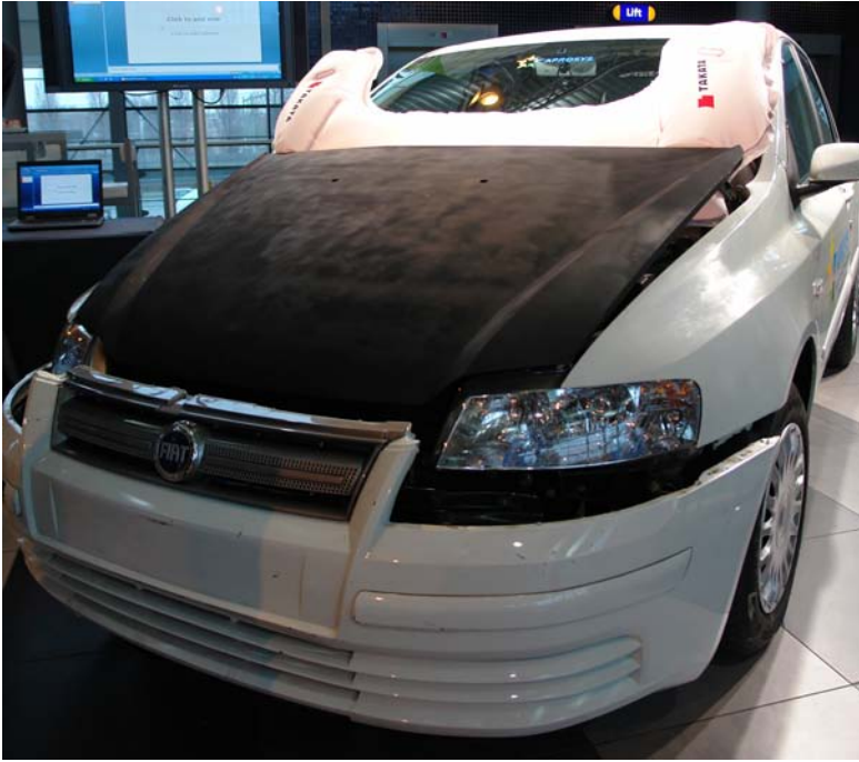
Figure 53. APROSYS project bumper and bonnet concepts for improved pedestrian protection. Project final event, February 2009.
