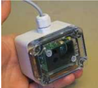
Figure 8. Road Eye sensor ( http://www.opticalsensors.se/roadeye.htm ). The dimensions of the casing are 51 × 53 × 45 mm.
