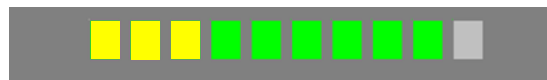
Figure 39. A bar graph concept showing friction levels. Yellow represents friction used, green is friction available (up to friction potential) and gray is used to fill the bar to a maximum value 1.0.
