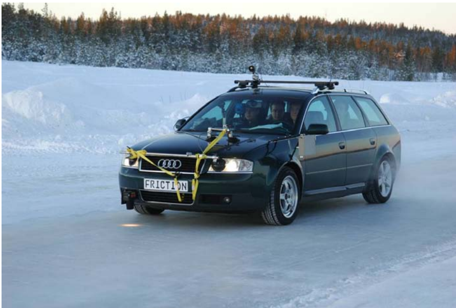
Figure 35. The development vehicle of the study, Audi A6, equipped with extra sensors and running a test program in Ivalo, Finland, 2007.
