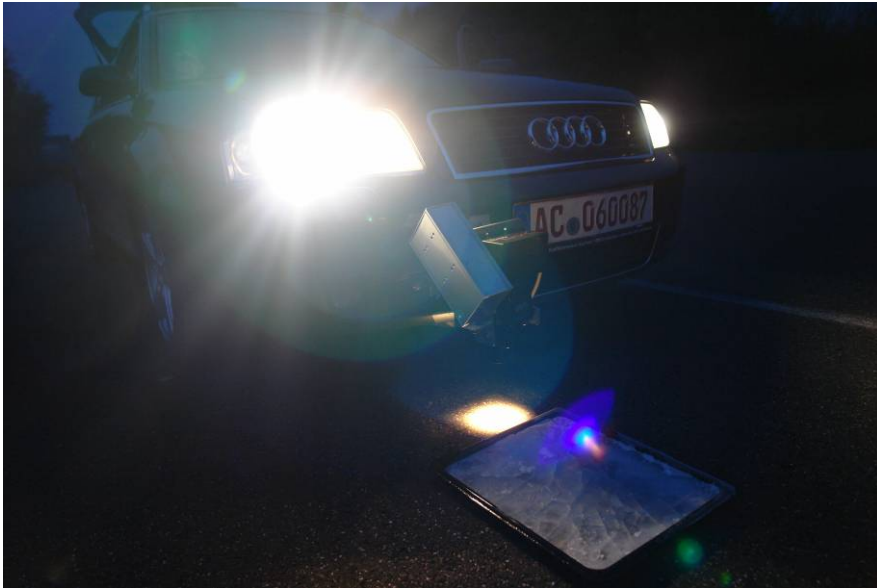
Figure 47. Night-time test of environmental sensors, especially ice detection. Aachen, October 2008.
