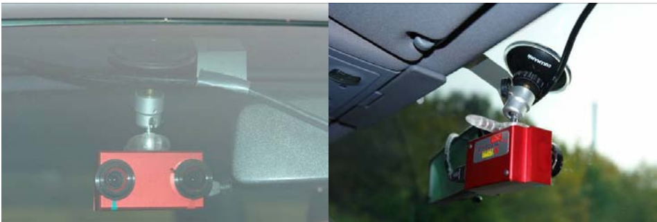
Figure 12. IcOR camera prototype with dedicated polarization filters.
