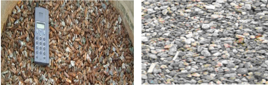
Figure 22. End products of sink-float process (left sink product, right float product).
