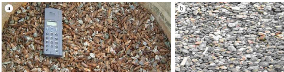
Fig. 4. End products of sink-float process (left sink product, right float product).
