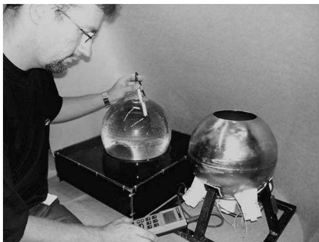
Fig. 1. Ultrasonic reactors constructed in this study.
