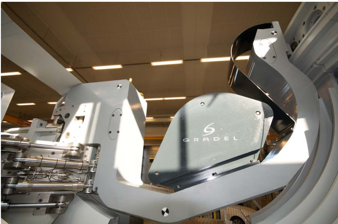
Figure 7.2. Divertor cassette entering the second cassette position.
