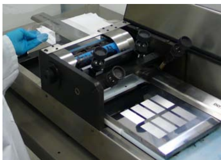
Figure 9. Pictures of two laboratory-scale gravure printing machines that have a) a printing plate (Norbert Schläfli Maschinen/Labratester) or b) a printing cylinder (IGT Testing Systems/IGT G1).
