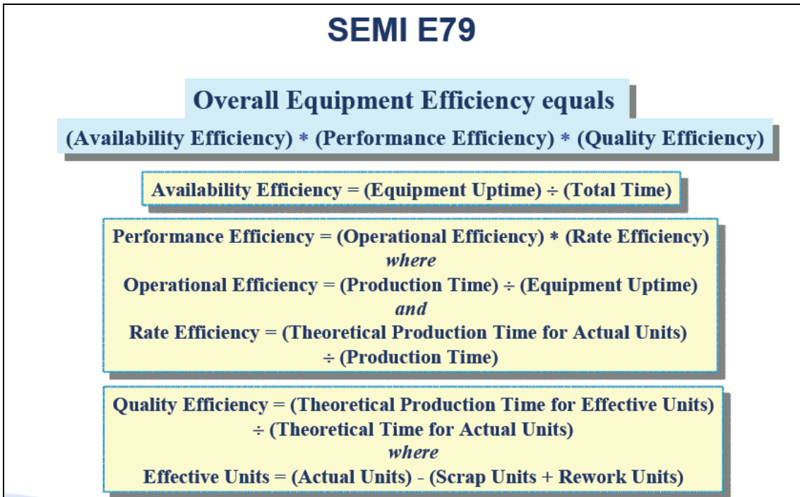
Figure 4. SEMI E79 formulas for computing the Overall Equipment Effectiveness (OEE).
