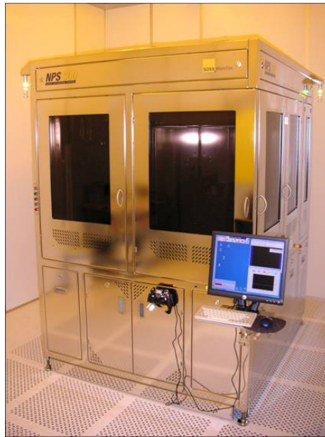
Figure 11. Photograph of the NPS300 nanoimprinting stepper in a clean room.
