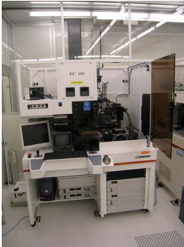
Figure 9. Photograph of an FC150 Flip Chip Bonder in a clean room.
