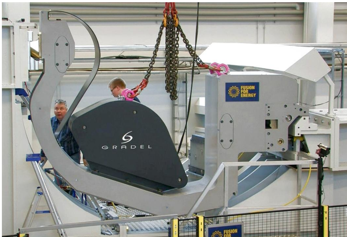
Figure 7.4. Test arrangements in the Divertor cassette locking tests.
