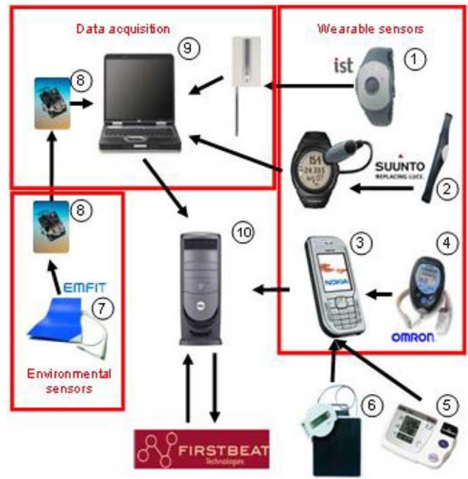
Fig. 1. Data collection equipment (details in text): (1) IST wrist activity monitor (actigraph). (2) Suunto HR monitor. (3) Nokia mobile phone with Wellness Diary application for self-assessments and measurement results from (4) Omron step counter, (5) Omron blood pressure monitor, and (6) weight scale, (7) Emfit bed sensor, (8) environmental sensors, (9) laptop PC, and (10) central server. Collected HR data were processed with Firstbeat PRO WAS.
