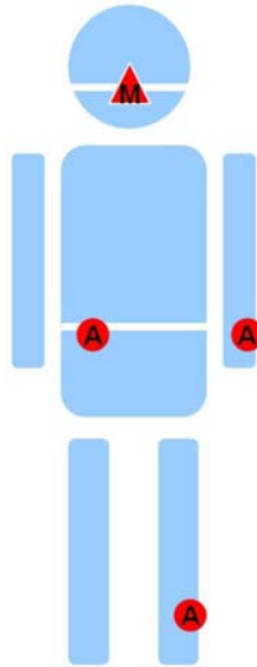
Figure 16. Study 3 data acquisition system: 3 data loggers (A) with a 3D accelerometer and 3D angular rate sensors on the body and the reference (M), a portable breathing gas analyzer.
