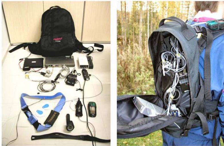
Figure 13. Study 1 Data Acquisition System: on the left: equipment on the floor, on the right: equipment in the rucksack. On the left, top row: Rucksack. Second row: PC battery, PC, Embla recorder (white) and battery. Third row: Oximeter (gray), SoapBox (black), microphone and amplifier (black), SensorBox. Fourth row: Respiratory effort strap (blue), body position (blue, around strap on the left), ECG electrodes (white-blue), skin temperature (silver, on top of the blue strap), skin conductance (gray, around the blue strap), Suunto wrist-top computer and its heart rate strap below, second oximeter (black), GPS navigator.
