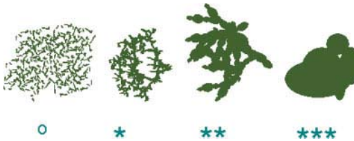
Figure 1. Classification of the ash residues with increasing sintering, as seen under microscope [14]. [Color figure can be viewed in the online issue, which is available at www.interscience.wiley.com .]
