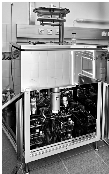
Figure 5. During this thesis VTT invested in a new SUNALE R-200 ALD-reactor which is not limited by clean room conditions.
