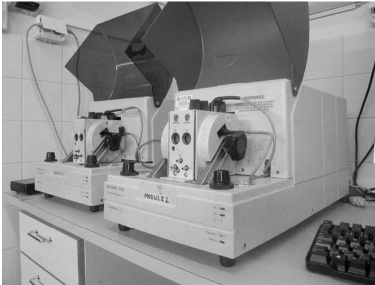
Figure 2. Equipment employed in measuring oxygen transmission rates.
