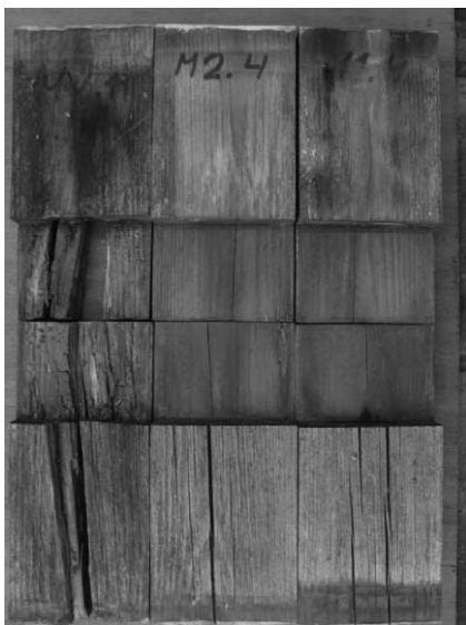
Figure 6. Pine samples (from the left: untreated, thermally modified at 210°C and 195°C) after 9 years of exposure. The upper and bottom sides of the specimens are at the bottom and top of the figure, respectively.
