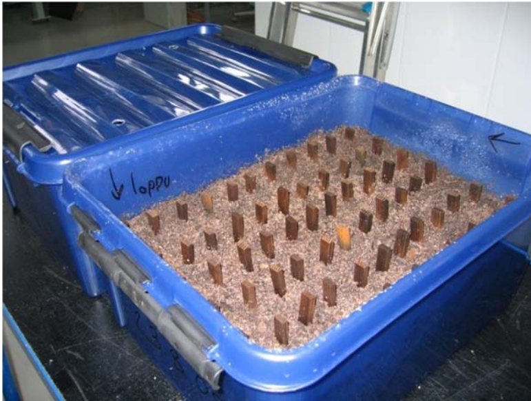
Figure 11. The specimens were incubated in containers in the soft rot test.
