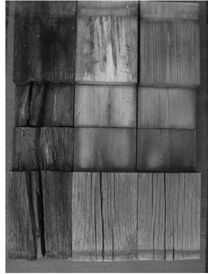
Figure 7. Pine samples [from the left: untreated, tributyl tin oxide (TBTO) and copper, chromium and arsenic (CCA) treated] after 9 years of exposure. The upper and bottom sides of the specimens are at the bottom and top of the figure, respectively.
