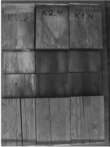
Figure 5. Spruce samples (from the left: untreated, thermally modified at 210°C and 195°C) after 9 years of exposure. The upper and bottom sides of the specimens are at the bottom and top of the figure, respectively.
