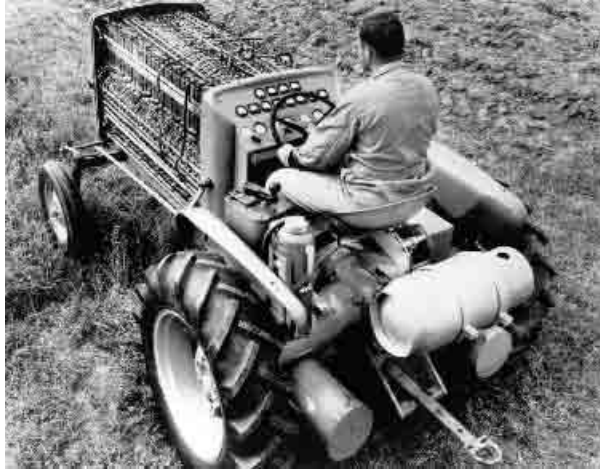
Figure 1. An experimental Allis-Chalmers fuel cell tractor in 1959 [7].
