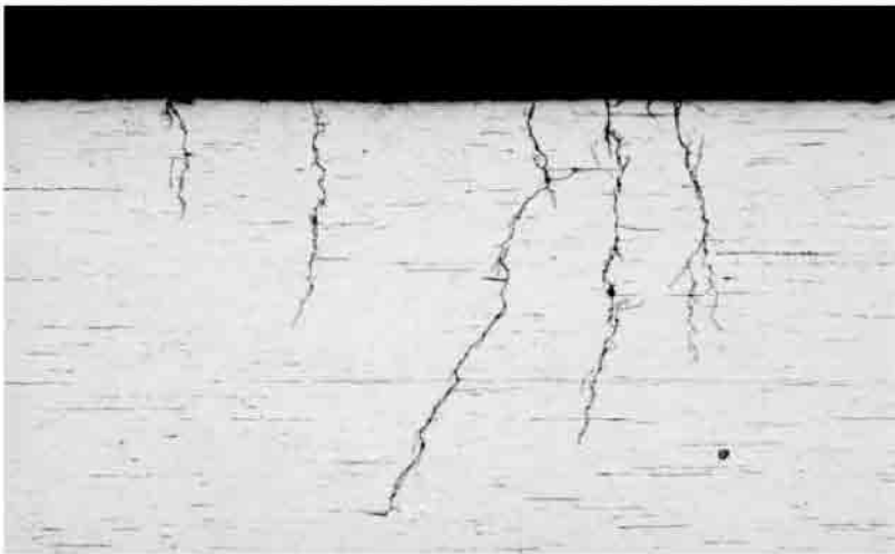
Figure 3.4-1. Microscopic detail of SCC in a steel component, from ref. [3].
