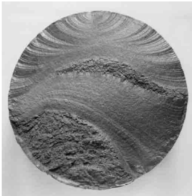
Figure 3.3-1. Fatigue damage of a shaft component, from ref. [3].
