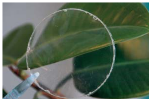
Figure 1. A transparent and flexible film obtained from a butylated and allylated xylan (left). Etherification routes using epoxy reagents in alkaline conditions(right): (i) xylan is first hydroxypropylated using propylene oxide and then (ii) further etherified using butyl and/or allyl glycidyl ethers; (iii) xylan is only etherified using butyl and/or allyl glycidyl ethers. (1) Hydroxypropylated (HPX); (2) hydroxypropylated and butyl-allylated (HPX-BA), and (3) butyl-allylated (X-BA) xylans.
