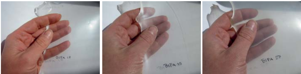
Figure 2. Biaxially oriented PLA-montmorillonite -nanocomposite films: BIPA18, BIPA19 and BIPA 27, from left to right.
