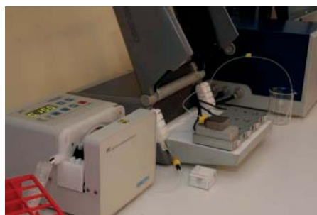
Figure 2. QCM-D instrument equipped with the humidity module (left) and a schematic drawing of the principle of the humidity chamber (right).
