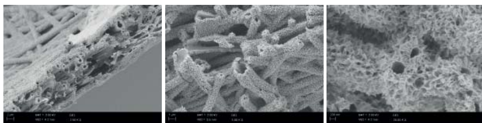
a) b) c) Figure 3. Nano-coral obtained using dissolution in the removal of the PVA template.
