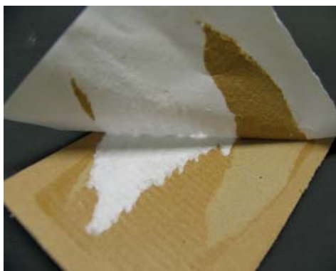
Figure 5. Gluing of cardboard using a water-based starch adhesive.
