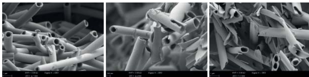
a) b) c) Figure 5. Nanotubes obtained by thermal decomposition of a) PVA b) PA and c) PVP.
