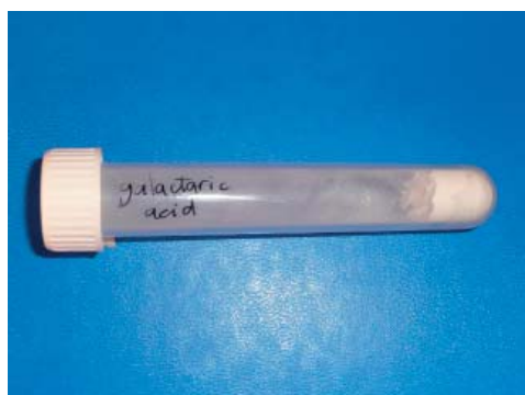
Figure 4. Galactaric acid produced from D-galacturonic acid by Hypocrea jecorina , purified by acid precipitation 6 .
