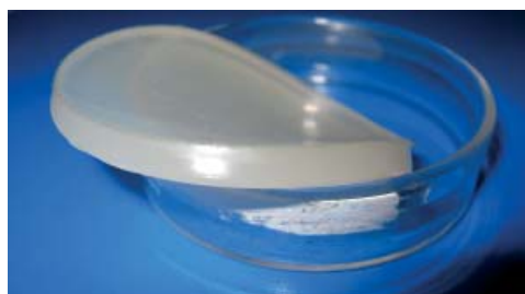
Figure 3. A hydrogel prepared from the allylated hydroxypropyl xylan (HPX-A) using 5 wt% of diallylarabinardiamide (DAD) straight after cross-linking in a UV oven.
