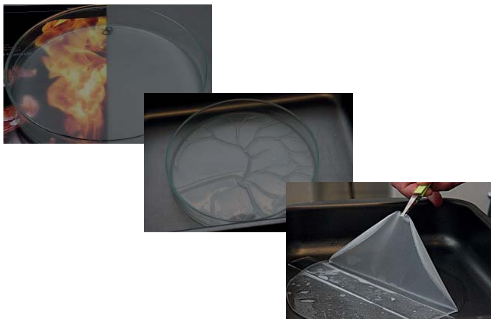
Figure 7. A stimuli-responsive membrane prepared from allylated cellulose fibres grafted with PNIPAM.
