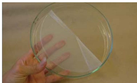
Figure 6. Allylated cellulose fibres cross-linked to a soft hydrogel-like membrane without any additional cross-linker or without grafting.
