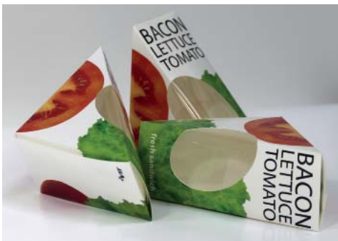
Figure 1. Bread package for daily use with a hemicellulose-based transparent window.
