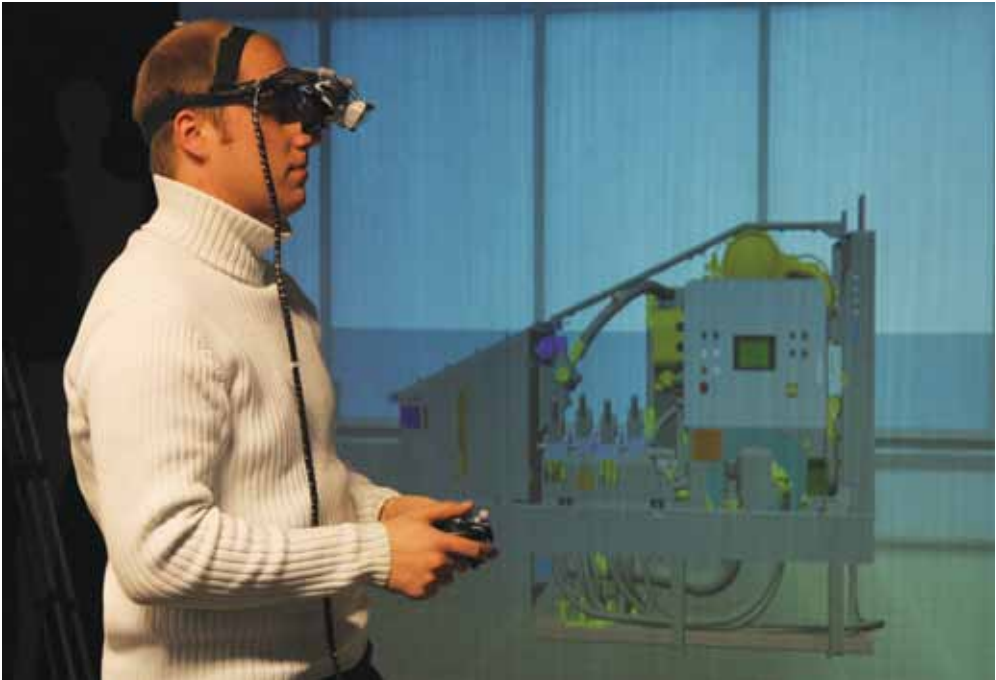
Figure 2. An example of the combined ManuVAR tool – participatory cross-disciplinary design review of a new product. Several experts – engineers, workers and managers – investigate a shared virtual environment view of the product (assembly sequence, ergonomics issues) before it is brought into production to find possible design faults. Source: [13]
