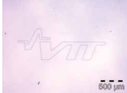
Figure 3. Transparent conductive ITO thin film patterned with a picosecond range laser without damaging the underlying glass surface.
