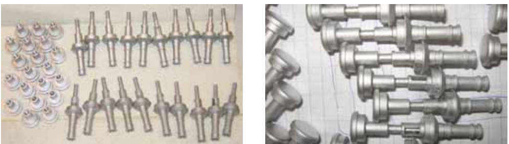
Figure 2. Moulded and sintered MIM counterparts. The male and female threads fit together perfectly.
