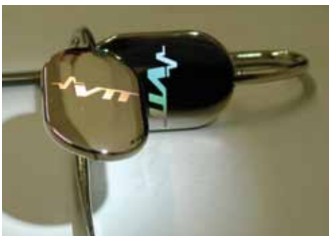
Figure 1. VTT logo made with grating-like structures.
