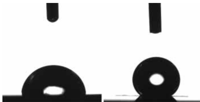
Figure 2. Contact angle measurement of the stainless steel surface. The value of 80^\circ is obtained for the smooth surface and 152^\circ for the structured surface.
