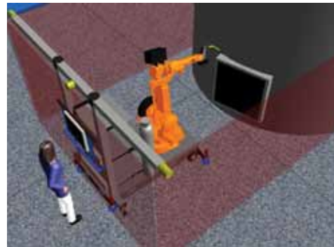
Figure 2. A conceptual picture of a freely transformable robot platform used in a welding application.
