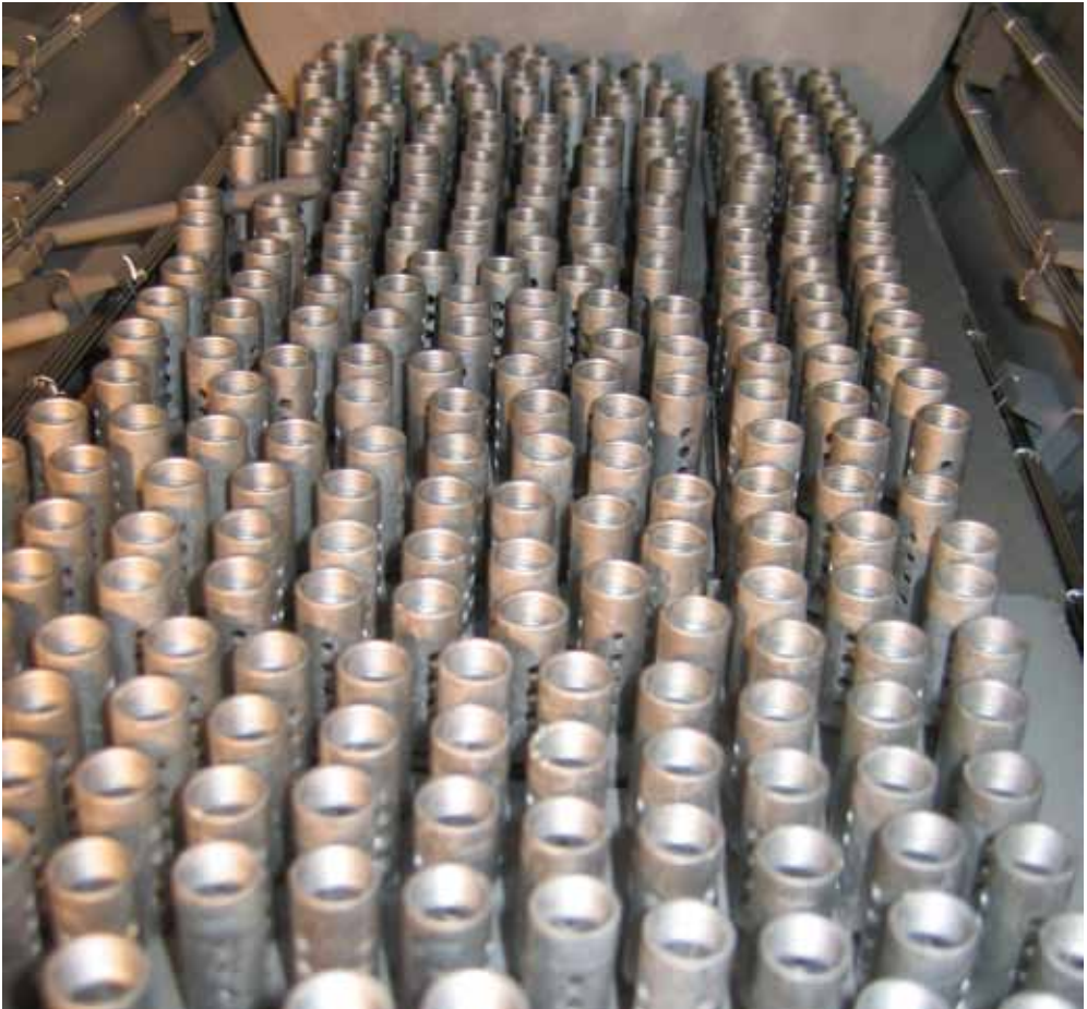
Figure 1. Sintered MIM components of stainless steel in the sintering furnace.
