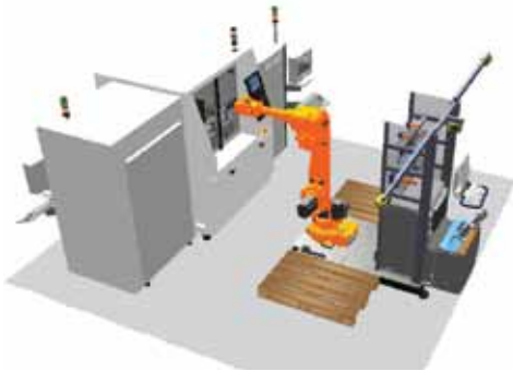
Figure 1. A conceptual picture of a transferable universal robotic platform for the material handling of machine tools.
