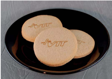
Figure 1. Direct marking methods offer potential for security marking and promotional marking on edible products. Left: laser marking on biscuits. Right: inkjet printing on pharmaceutical capsules (photographs by Heidi Eriksson and Liisa Hakola).
