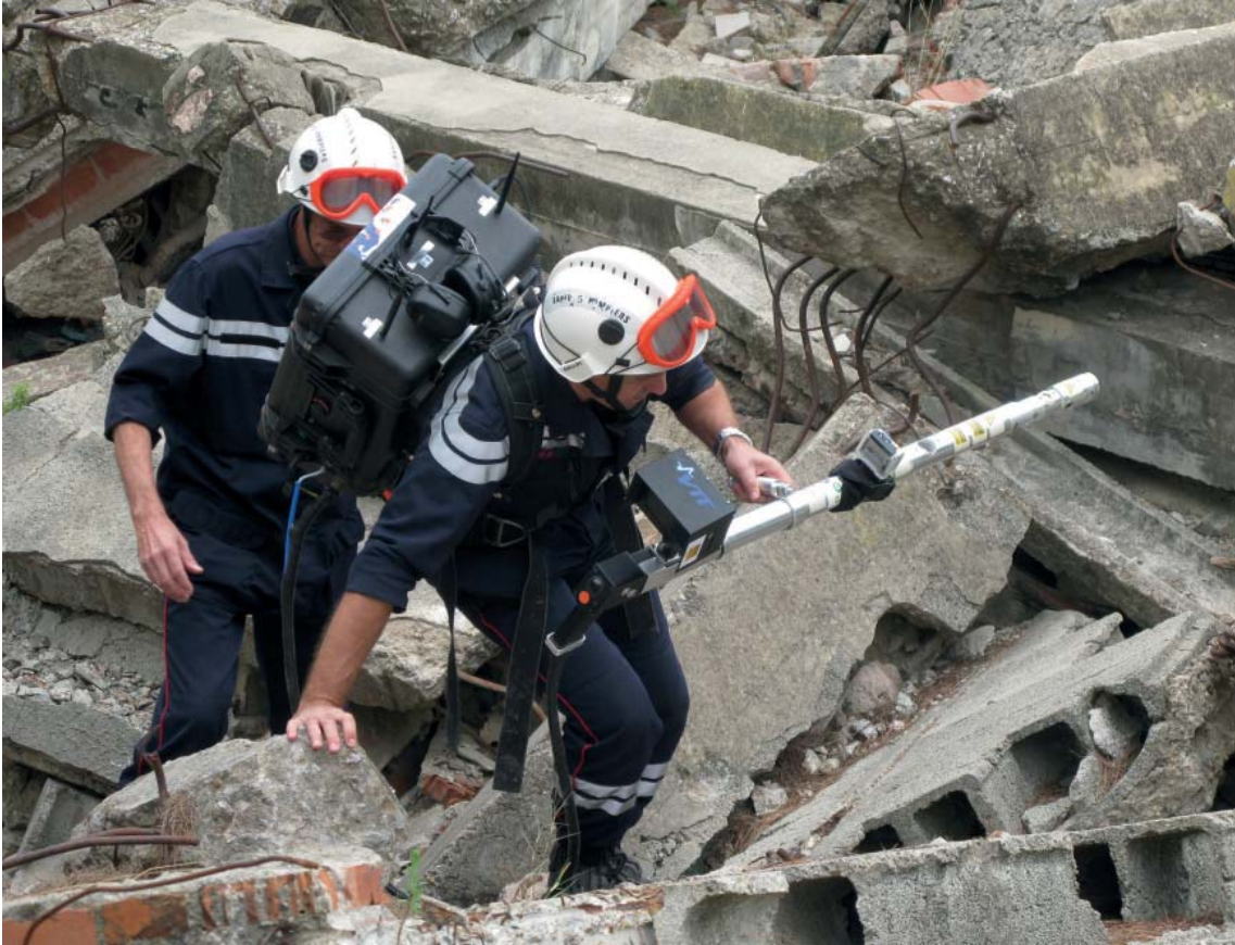
Figure 1. FIRST responder device being tested in the Gava test field.
