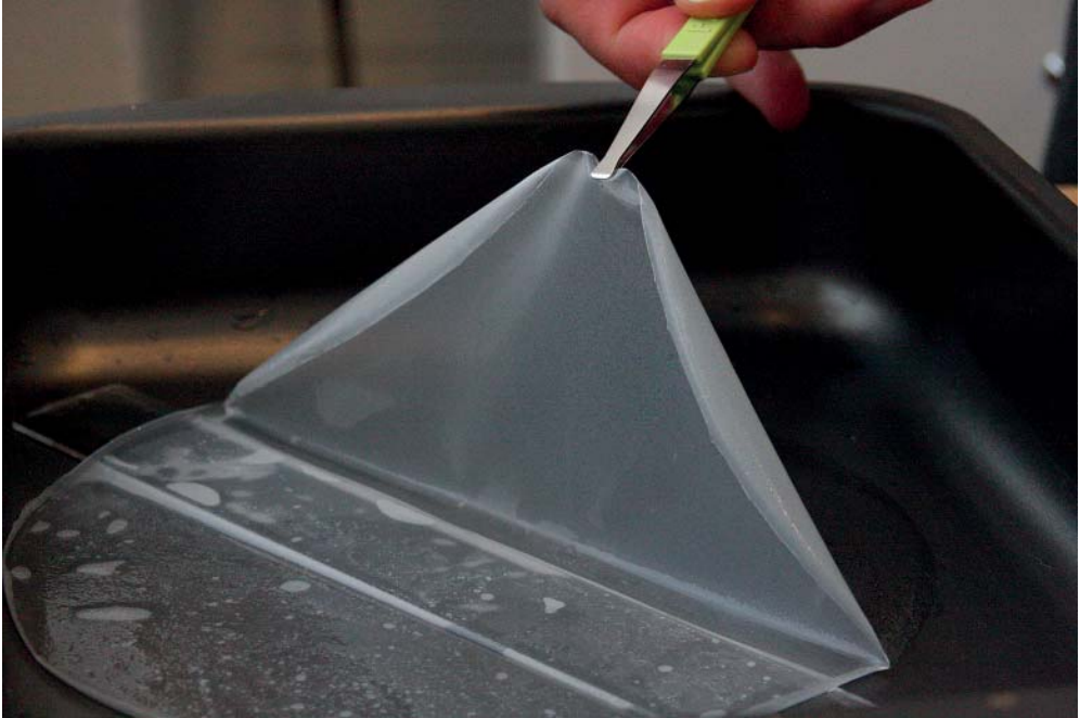
Figure 2. Thermo-responsive cellulose-based membrane. Bio-based membranes decrease the need for material produced from fossil resources, thus supporting sustainable development.
