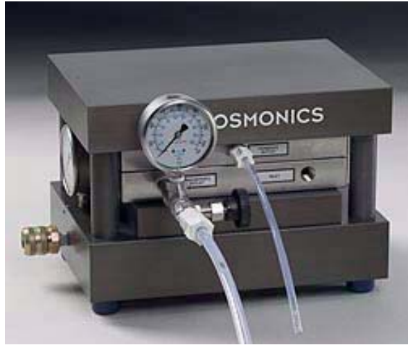
Figure 3. Equipment and a module for reverse osmosis research for e.g. desalination solutions.
