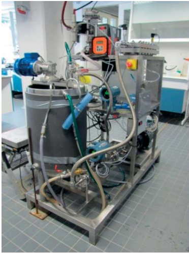
Figure 3. Equipment and a module for reverse osmosis research for e.g. desalination solutions.
