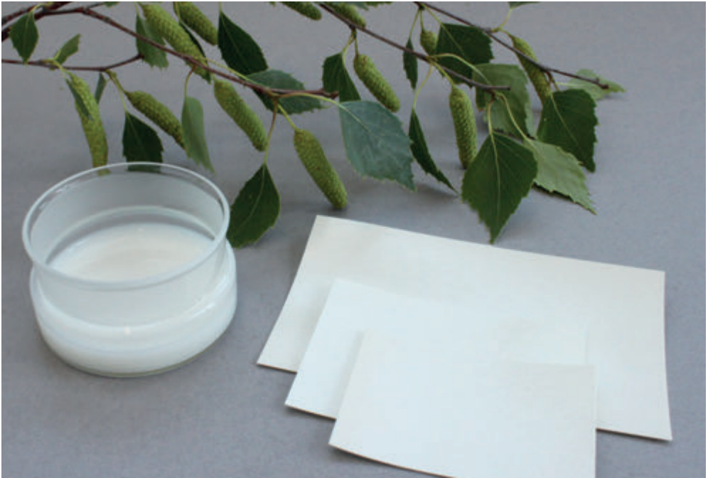
Figure 1. Bright white suspension of purified (desalted) xylan(left) and barrier coating on precoated board (right).
