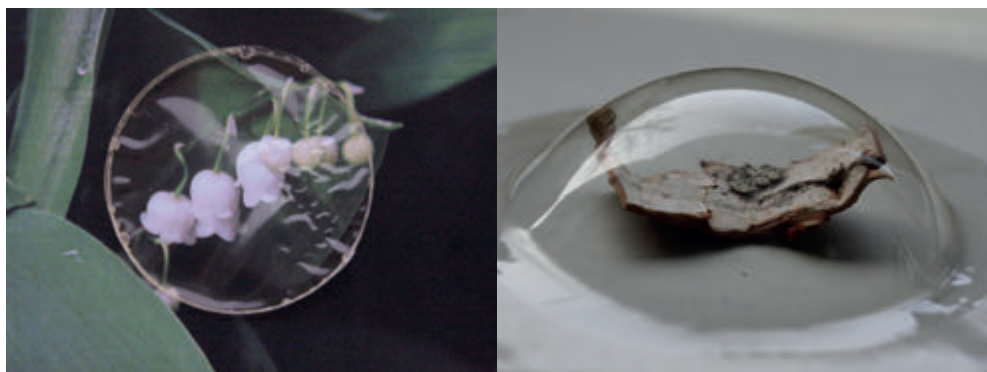
Figure 4. A transparent and flexible film obtained from a butylated and allylated xylan (left). Thermo-formable film produced thereof (right).
