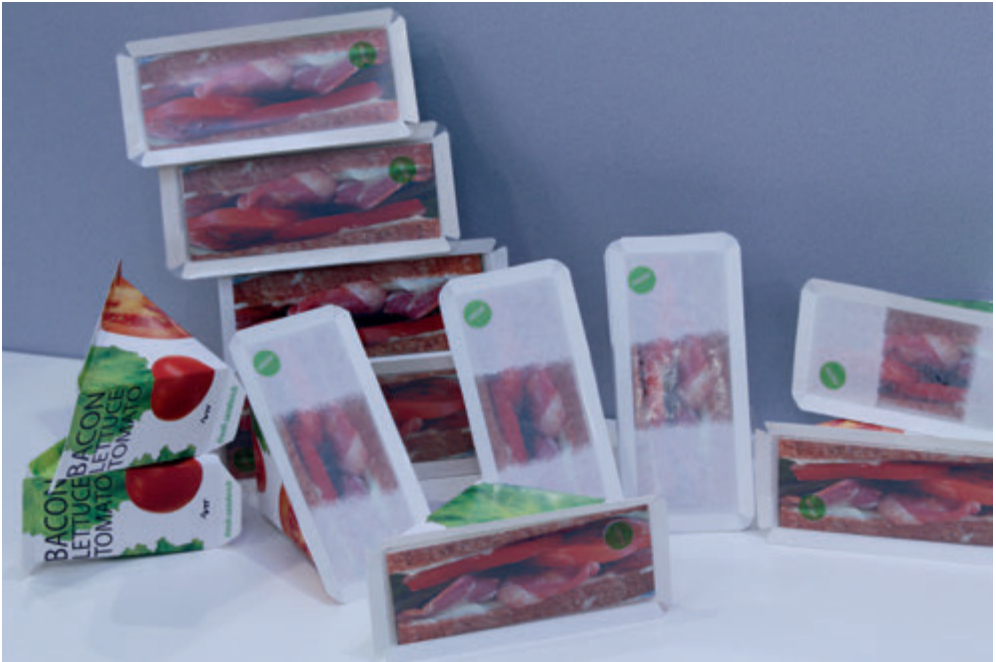
Figure 11. PLA films in sandwich packages as an option, among other bio-based package covers.
