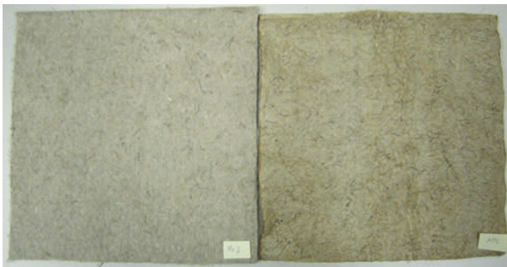
Figure 4. Untreated and APS-treated fibre mats used for thermoset composite reinforcement.
